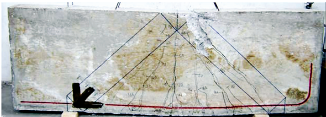
Figure 3 - Experimental failure and predicted numerical failure for specimen DB1.0-0.75 (figure only shows crack widths over 0,5 mm)
