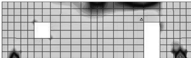
Fig. C—Principal compression stress for deep beam.
